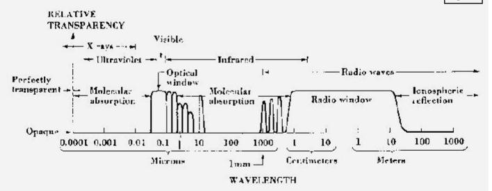
Figure 1. The electromagnetic spectrum showing relative transparency of the earth's atmosphere and ionosphere. (From Kraus, <u>Radio Astronomy</u>, 1s edition, 1966, p. 2.)
