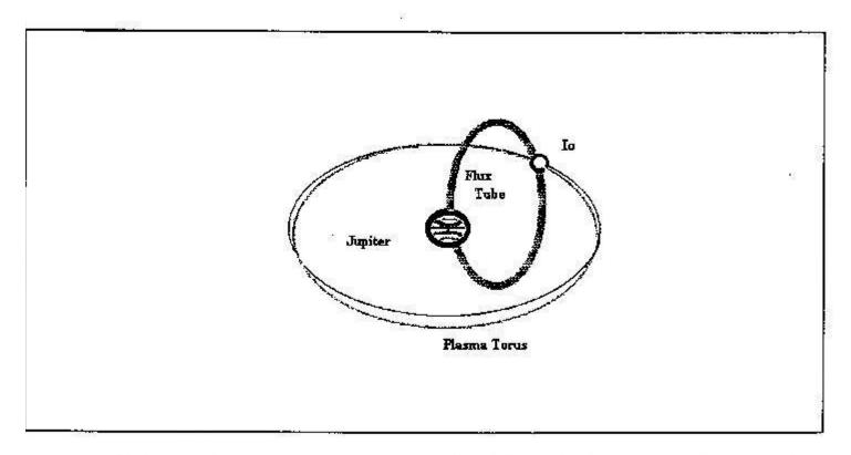
Fig. 21 I.4 This sketch illustrates the toroidal shaped plasma distribution around Jupiter and the orbit of Jupiter's moon, Io. The toroid is slightly inclined relative to Io's orbit because of the influence of Jupiter's strong magnetic field on the charged particles. The flux tube shown linking Jupiter and Io carries a current of about 5 million amperes.
