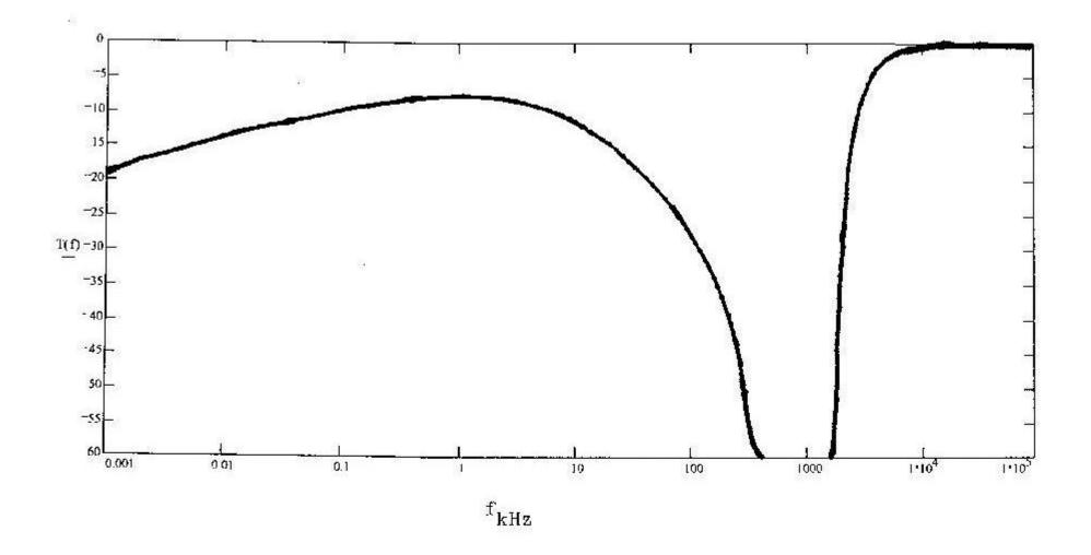
Fig. 5.4 Night-time Extraordinary wave ionospheric transparency for frequencies from 1 Hz to 100 MHz during a solar minimum. (The horizontal scale is in kHz.) Note that even under the best of conditions the ionospheric transmissivity in the 200 kHz to 2 MHz region drops below -60 dB.
