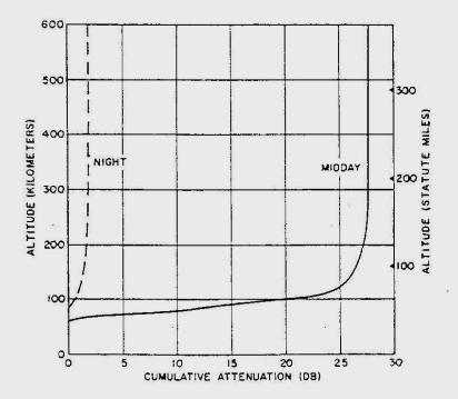
Figure 6. Minimum possible transmission loss (least possible attenuation) of an 18 kHz radio wave passing vertically upward through a standard model ionosphere versus altitude. (From Leiphart et al, 1962.)
